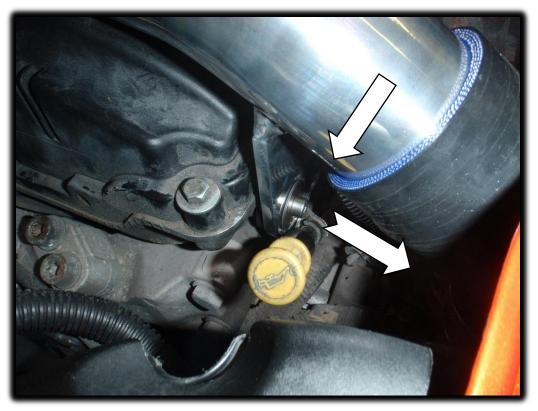
6. Once the inlet boost pipe is fitted and secured attach the boost outlet again using bolts and washers supplied.
