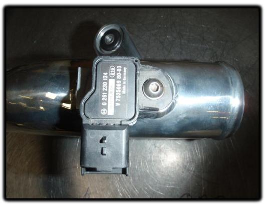
4. Fit the boost inlet pipe first as the bolt by the dip stick is hard to get too, use the bolts and washers supplied in the kit.
